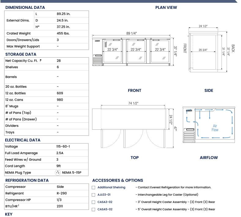
(†) Based on evaporating temperature of 23°F (-5°C) & condensing temperature of 131°F (55°C). (►) Product capacity is calculated based on standard industry figures. (※) Reference plan view for clarification on caster/unit height. If dimensions and capacity are critical, please contact Everest Refrigeration. Blizzard R290 replacement is at the sole discretion of Everest Refrigeration. Specifications subject to change without notice.
